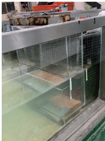
Figure 5. The water level line inside the U-OWC chamber.
