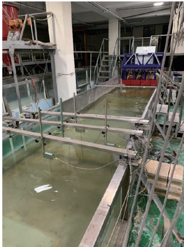
Figure 2. Displacement piston wavemaker and the wave tank.
