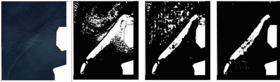
Figure 7. Comparison of the results of three modes to identify images under cloudy conditions (left to right: original image, U-Net, DeepUNet, VGG16UNet).
