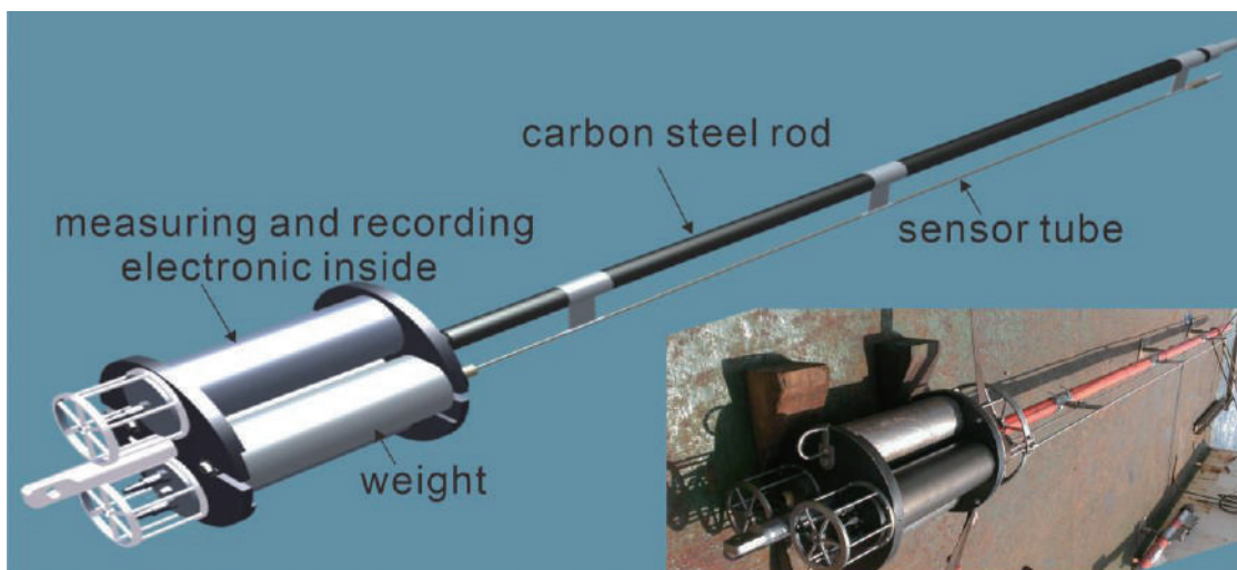
Figure 2. The instrument sketch and operating pictures of Lister-type Marine Heat Probes. (after Chen et al., 2019)
