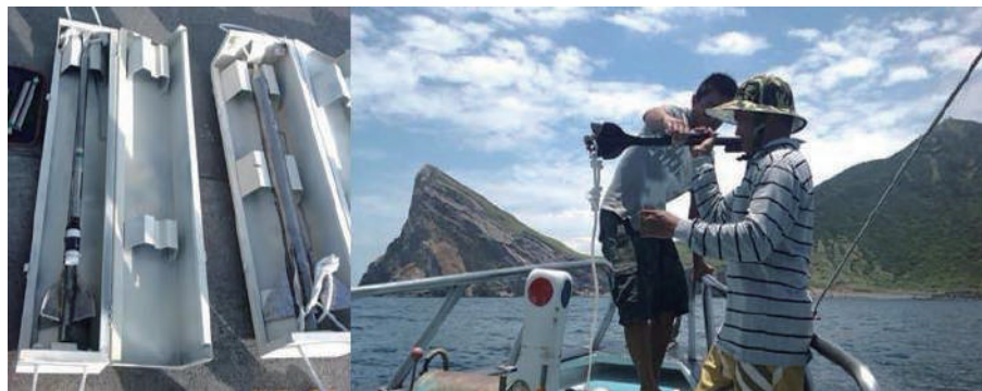
Figure 1. The portable miniature temperature loggers attached to a steel bar allowed us to use workforce to detect the seafloor temperature around Turtle Island. (after Chiang et al., 2008)
