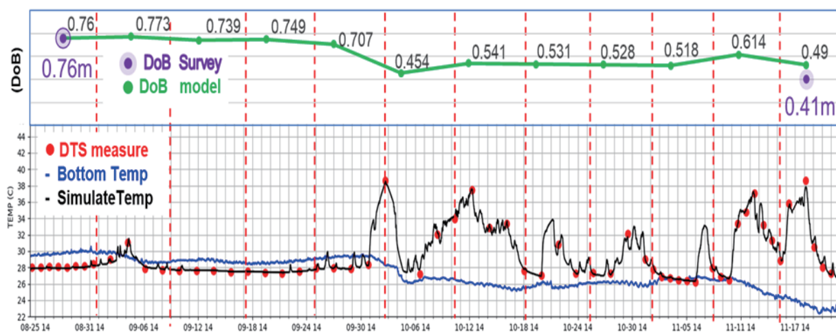
Figure 14. Simulation results of temperature and burial depth variations at the fiber optic section of the submarine cable in Area A.
